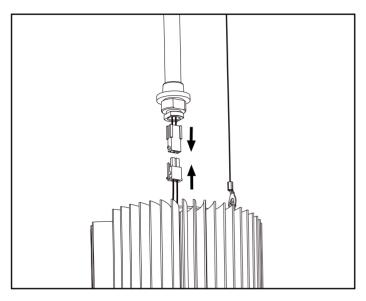
Step 5 Connect the electrical connections.
