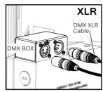
ed Connect DMX by using a standard DMX512 XLR cable with 5 pin in/out connector (by others).
