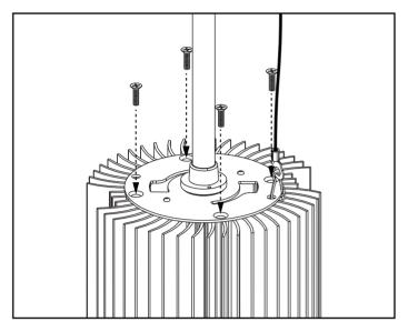
Step 5 Pull down the conduit wire and plating on top of the engine and screw 4 Phillips screws on top of the light engine.
