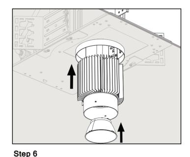
Install the reflector on the LED holder in the light engine. Bring the light engine back into the bracket.
