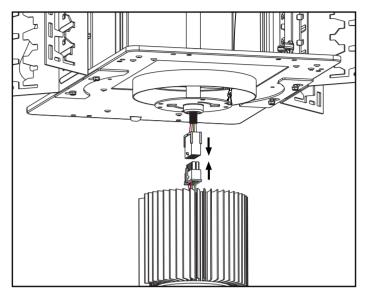
Step 4 Connect the electrical connections.
