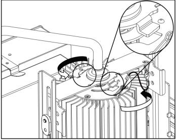
Step 7 Adjust the light engine into the support and slightly turn it to the right to secure it.
