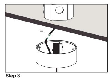
Connect the wires according the WIRING DIAGRAM provided.
