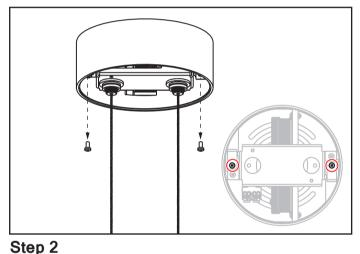
Unscrew the Phillips screws as indicated to remove the crossbar.
