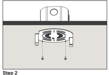
Screw the crossbar to the desired place on the ceiling and screw in place.
