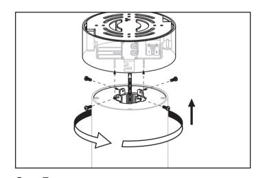
Step 7 Align and twist clockwise to lock the fixture in place. Screwing four sides to secure.
