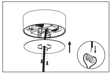
Bring up the canopy to the surface mount plate and screw in the screws set aside in step 2. Connect the DC wire between the fixture and canopy.
