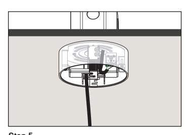
Step 5 Connect the wires according to the WIRING DIAGRAM.
