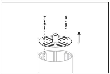
Remove 4 Phillips screws holding the fixture plate to adjust mounting height.
