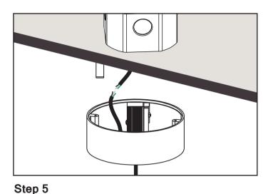
Make DC electrical connections to the fixture based on the wiring diagram.
