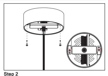
Open the remote power box, make AC and Dimming electrical connections based on the wiring diagram and close the remote power box.
