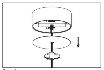
Step 1 Remove knockout and connect flexible conduit (not included).
