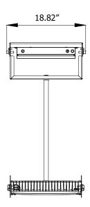
**Glare Shield Baffle**
