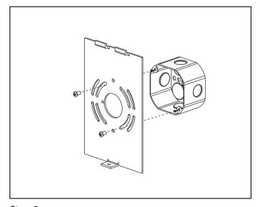
Step 2 Attach mounting plate to junction box with screws from junction box (by others).
