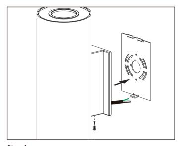
Step 1 Detach mounting plate from cylinder.
