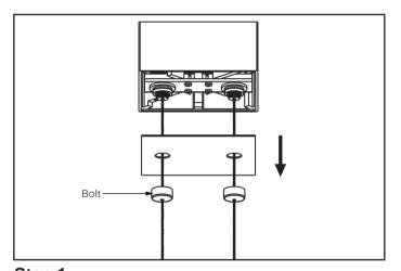
Step 1 Unscrew the 2 Bolts holding the Canopy Plate.
