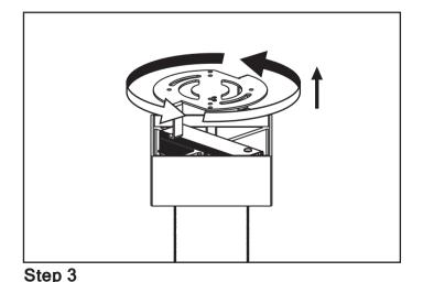
Twist the crossbar-anti clockwise to release it and set aside.
