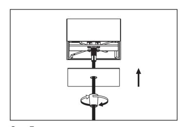
Step 7 Push the canopy plate up and secure it in place by tightening the cord grip clockwise.
