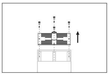
Step 8 Remove 4 Phillips screws holding the fixture plate and put aside.
