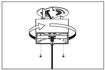
Step 6 Align the canopy to the crossbar and turn clockwise to lock it in place and screw in place.
