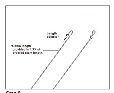
Step 8 Loop the aircraft cable through the mounting corners and tighten the clamp by adjusting the screw. Ensure that the height is adjusted before tigtening the clamp.
