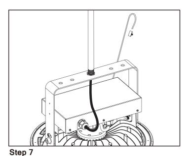
Clasp the hook onto the allocated bolt on the fixture mount.
