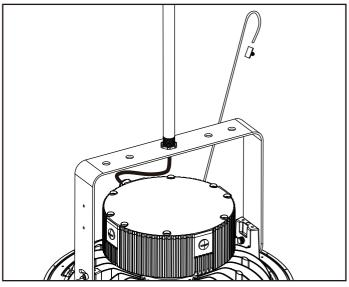
Step 7 Clasp the hook onto the allocated bolt on the fixture mount.
