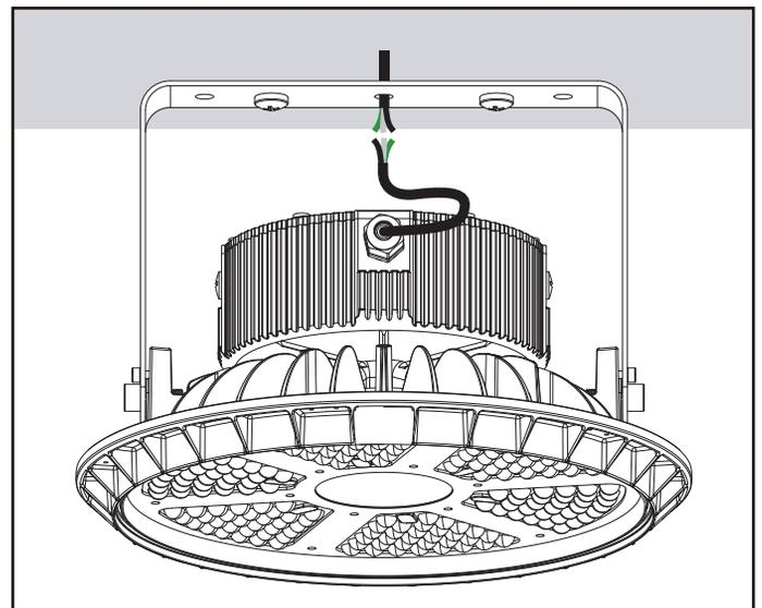
Make electrical connections between junction box and fixture.
