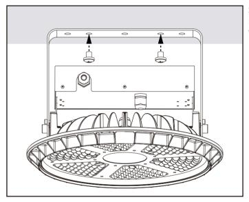
Secure mounting bracket to level surface with mounting hardware that is sufficient to support weight of the fixture.
