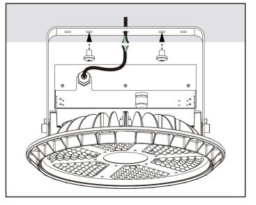
Make electrical connections between junction box and fixture. Refer to wiring diagram for a more detailed explanation.
