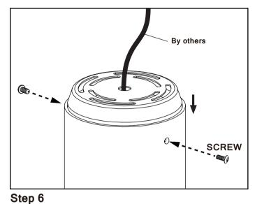
Fasten the lid and then Screw both sides of the fixture.
