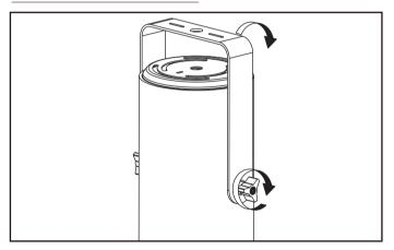
Step 1 Loosen the three arm knob to swivel the Yoke mount bracket to your desired location.
