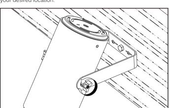
Adjust the desired angle and tighten the three arm knob to fasten the yoke mount in place.
