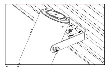
Step 2 Fasten the Yoke mount bracket on the desired location.
