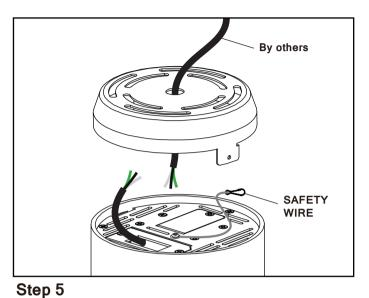
Connect the wires according to the wiring diagram on page 3.
