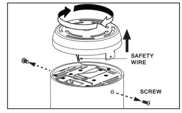
Step 4 Loosen two screws on the side of the fixture. Twist and lift up the lid from cylinder. Unhook the safety wire from cylinder to detach the lid.
