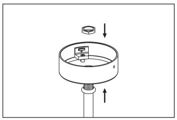
Step 6 Fasten the stem canopy to the stem by using a Hex bolt.
