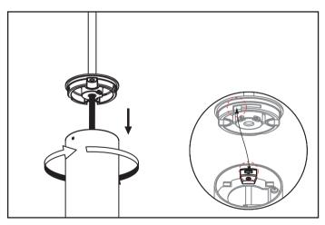
Align the bottom part of the fixture with the stem mount plate by matching the U-shaped openings.
