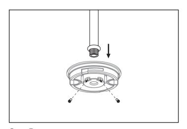
Step 5 Screw in the stem to the top fixture plate and lock it in place by using the 2 screws as indicated.
