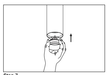
Step 7 Push back the trim and optics back into the fixture.
