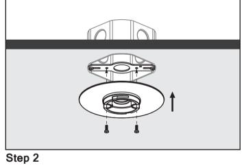
Screw the surface adjustable mount plate onto the bracket in the two holes indicated.
