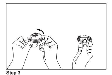
Facing down, push up on the optics from underneath until it slides out.
