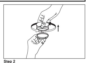
Turn the trim clockwise to unlock the lens holder.
