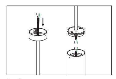
Step 7 Loop the wire through both ends of the stem, referring to the wiring diagram for connection to the fixture.
