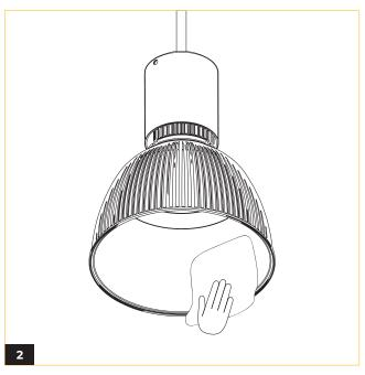
Clean the interior and exterior surface using a soft rag with
