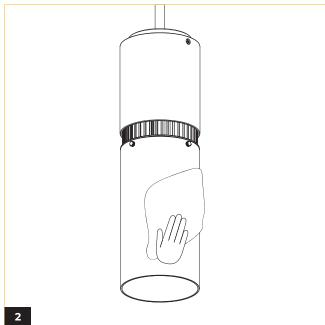
Bring up the diffuser to the fixture and align it to the indicated openings and fasten in place with 4 thumb screws.
