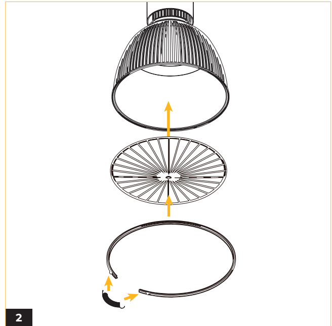
2 When specifying the conical lens accessory. Cover the shroud with the conical lens plate and fasten in place using the provided metal band.
