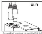
\*The last fixture has to be terminated with a DMX Terminator (by others).
