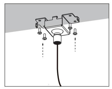
Step 2 Mount the mounting plate and swivel ball onto flat surface using screws.
