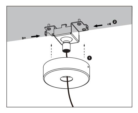
Step 3 Mount canopy onto mounting plate and lock in place
