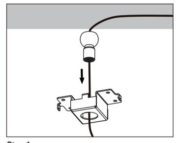
Step 1 Thread AC wires through swivel ball and mounting plate.
